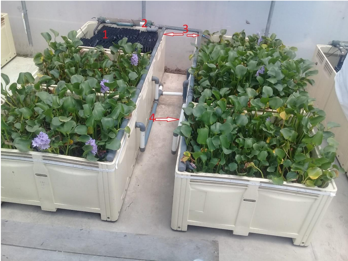
Figure 4.1: Arrangement of each flow through system where 1 = the feeder tank that supplies nutrient enriched water to the other 5 tanks in the series; 2 = the UV filter to reduce algal growth in the water supplied to the rest of the flow through system; 3 = delivery pipes from the feeder tank to the other tanks; 4 = return pipes from the other tanks to the feeder tank.
