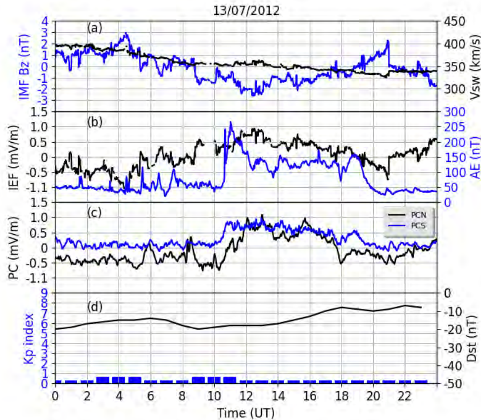
Figure 5.8: Variation of interplanetary magnetic field ( B_z [nT]), interplanetary electric field (IEF [mV/m]), AE index (nT), polar cap (PCN and PCS [mV/m]), Dst index and Kp index on 13 July 2012 ( https://omniweb.gsfc.nasa.gov/ ).
