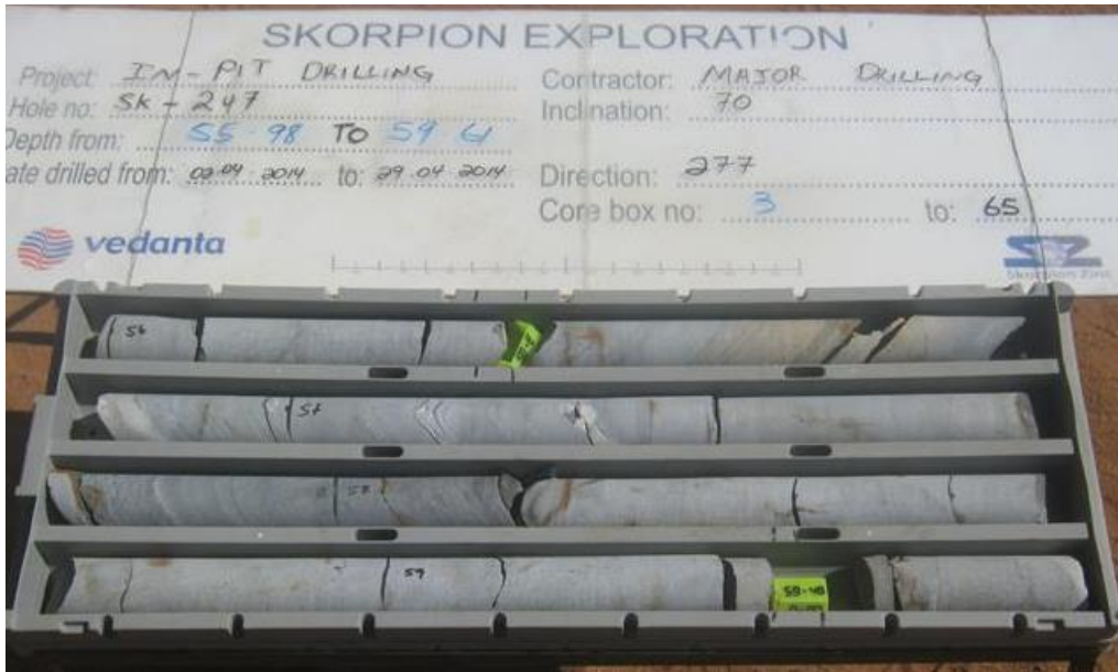
Figure 8: Core photo of the Skorpion limestone in a 1m HQ core box, the colour varies from light grey to dark grey limestone with varying content of \text{CaCO}_3 (this study, 2014).
