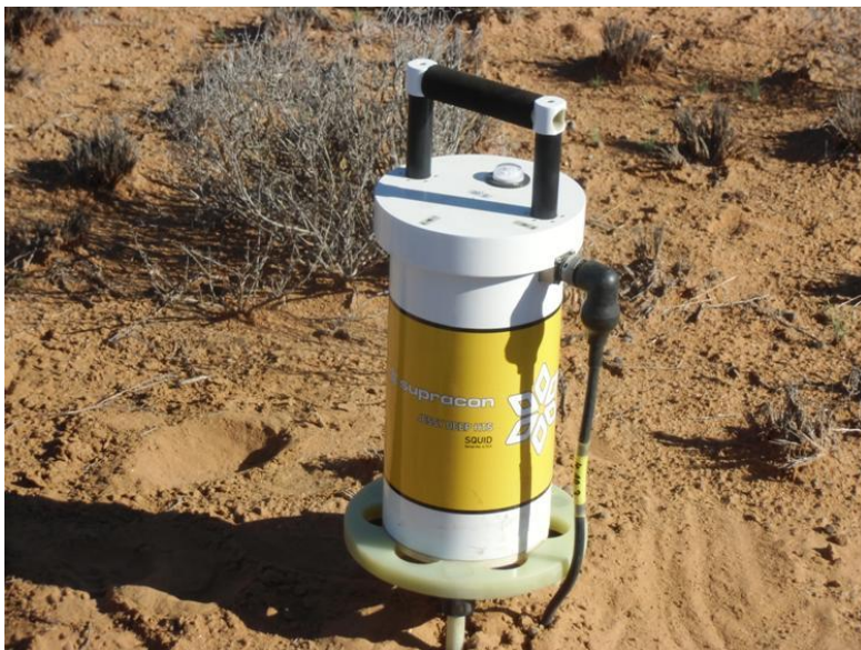
Figure 17: The HT SQUID magnetometer device used in the survey program. Picture taken during survey at Skorpion Mine (this study, 2014).
