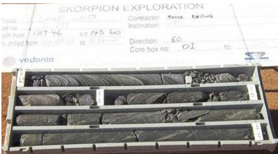
Figure 10: Core photo of the chlorite biotite schist in a 1m HQ core box, the dominant mineral in the mafic rocks units are mainly amphibole and biotite (this study, 2014).
