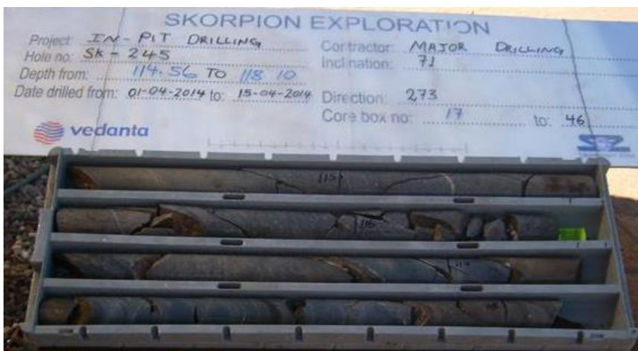
Figure 7: Core photo of the Skorpion arkose in a 1m HQ core box displaying intense fracturing usually filled with iron oxides (this study, 2014).
