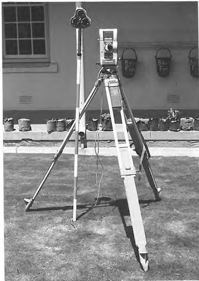
Figure 30 The Shokkisha electronic theodolite that was used to log the microtopographical data of the camps.
