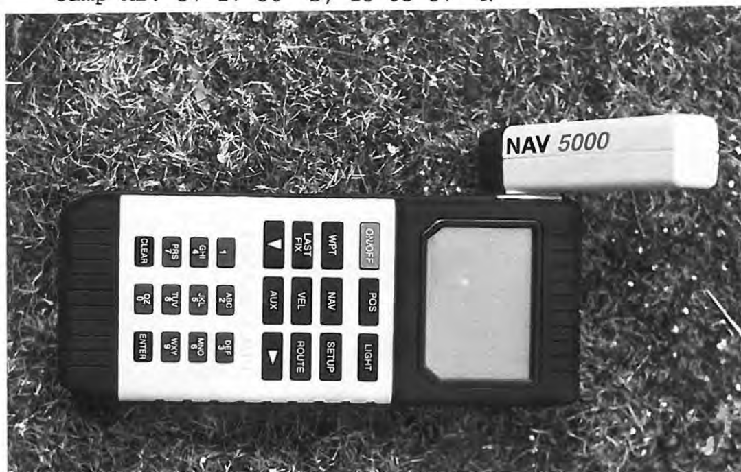
Figure 3 The Magellan GPS NAV 5000, handheld global positioning system, used to determine the geographical coordinates of the two Sites, A and B, and for camps DA, MA, DB and MB.
