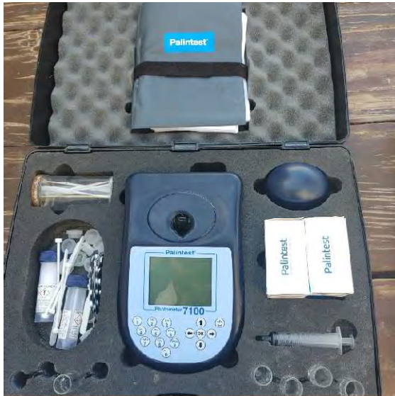
Figure 2.5: Image of the Palintest spectrophotometer along with the accessories used to determine ammonia concentration in the experiment tank system.
