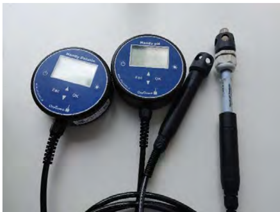
Figure 2.4: Image of the portable Handy Polaris (left) and Handy pH (right) instruments used to determine water quality by measuring temperature, pH, dissolved oxygen, and saturation.
