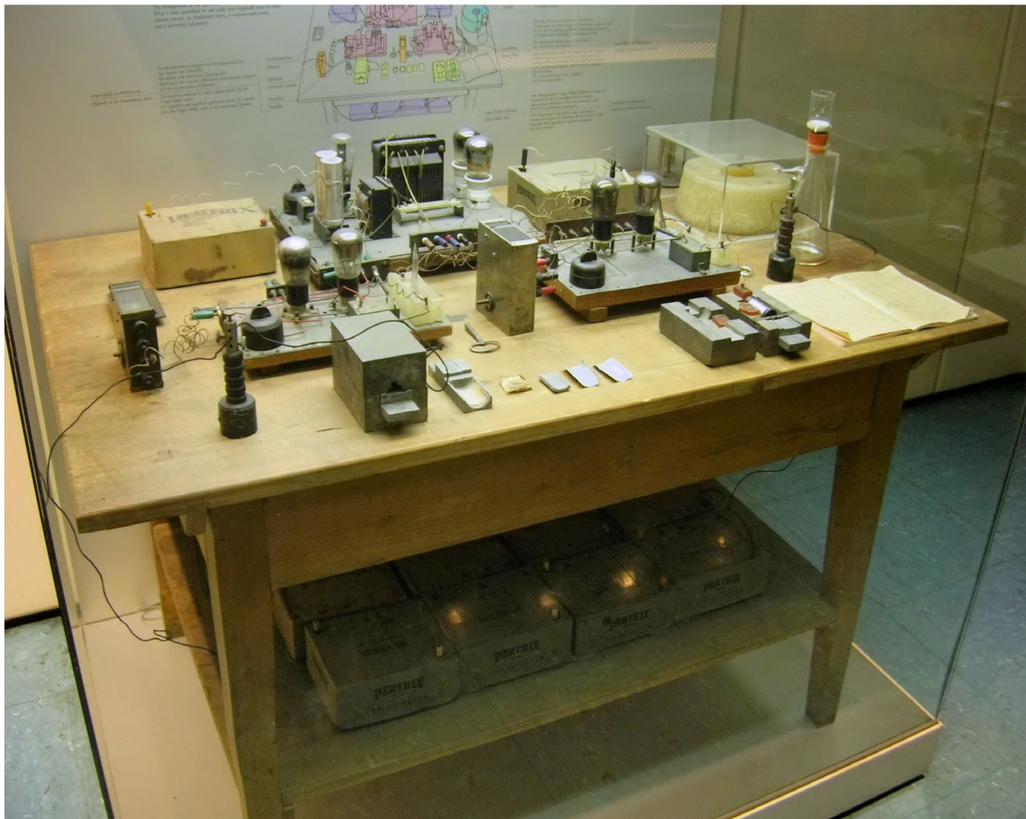
Figure A.1: The apparatus used by Otto Hahn and Fritz Strassmann for the discovery of neutron-induced fission of uranium in 1938 [41].
