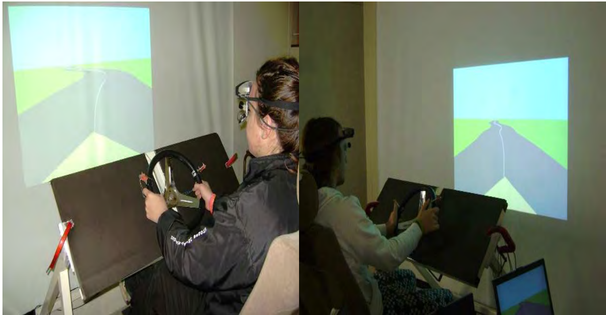
Figure 10: Participants wearing the head mounted eye tracker and performing the primary driving task.
