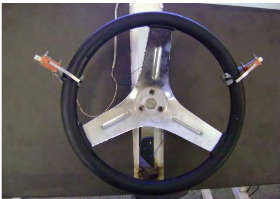
Figure 12: The two clickers located on the steering wheel for stimuli response.
