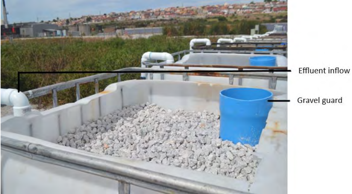
Figure 2.5 The top of an ebb and flow filter, with a view of the other filters connected next to it.
