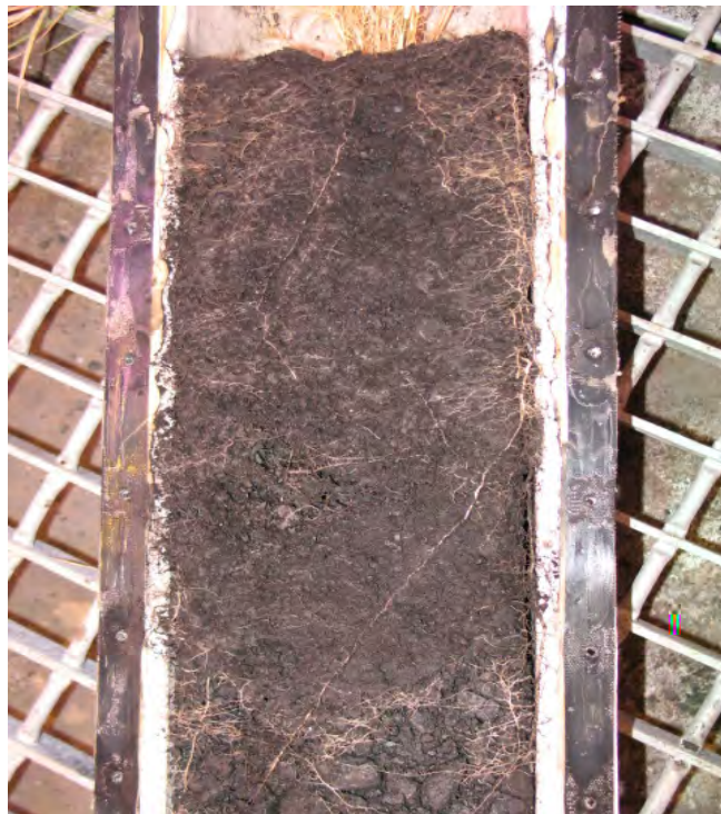
Figure 4.8. A close-up frontal view of the upper (0-40cm) section of a treated column in which the majority of root establishment took place.
