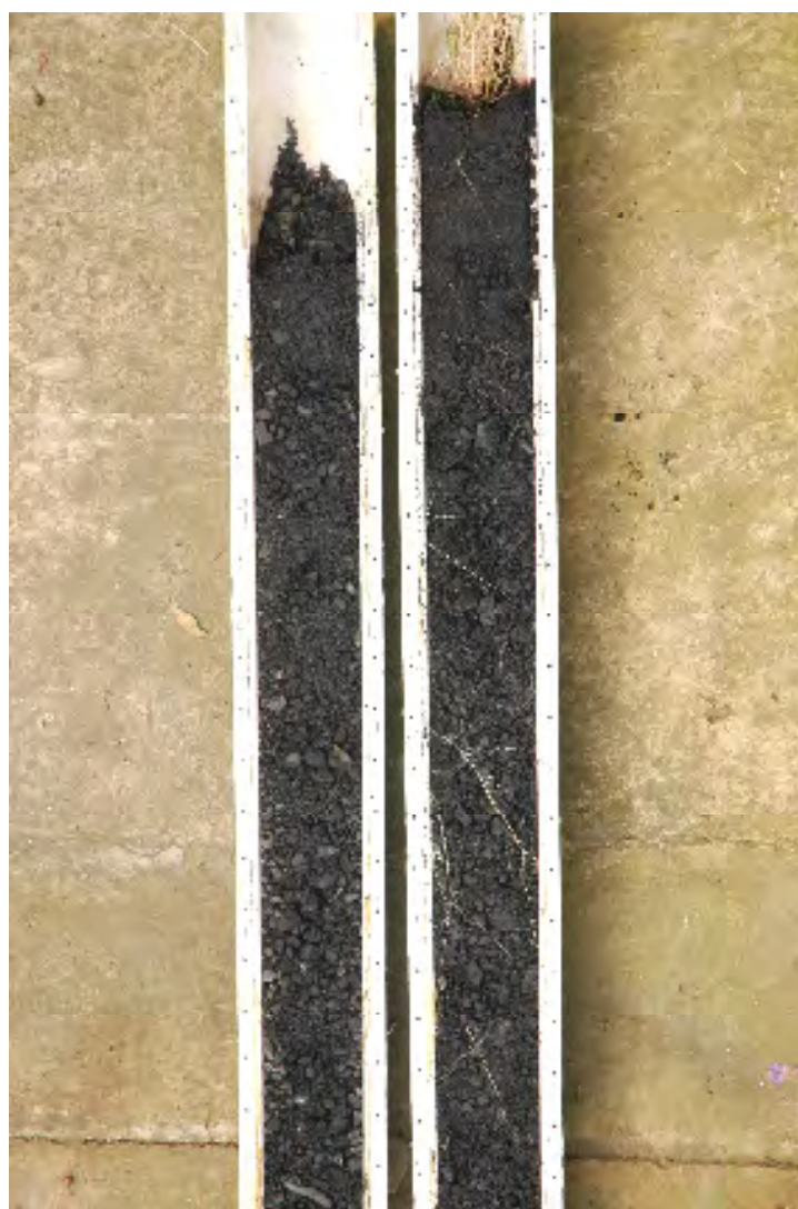
Figure 4.6. A longitudinal view showing root penetration in a column containing Cynodon dactylon (right) compared to a hard coal control column (left) after 44 weeks incubation.
