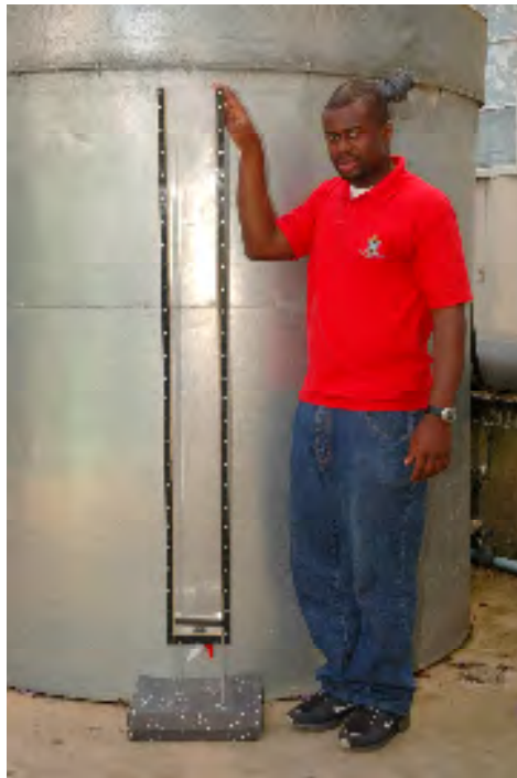
Figure 4.1. Frontal view of a column used in the coal dump simulation studies. Columns were constructed out of sturdy Perspex with a front cover screwed on. The author shows the comparative size of the column with dimensions of 1.50m height, 12.7cm width and 6.7cm depth.
