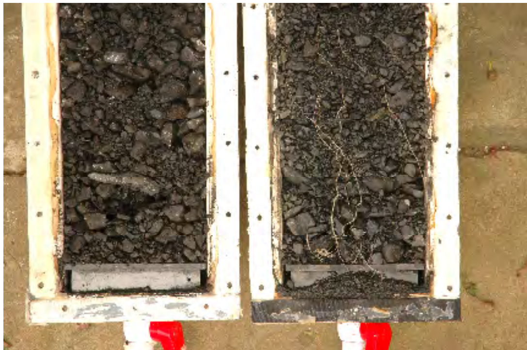
Figure 4.10. A close-up frontal view of the bottom sections of a treated column (right) compared to a hard coal control column (left) showing increased coal degradation.
