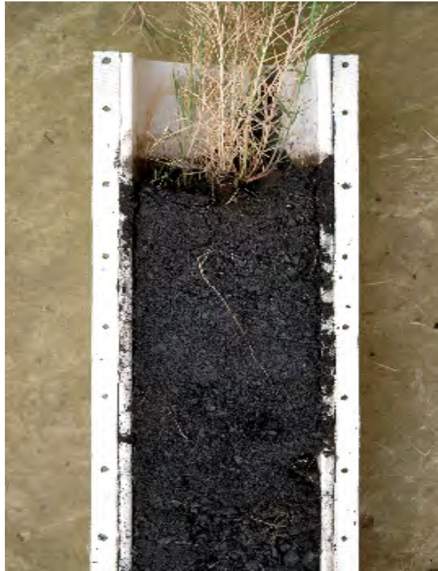
Figure 4.7. A close-up frontal view of the top 20cm section of a treated column planted with Cynodon dactylon showing breakdown of the coal substrate.
