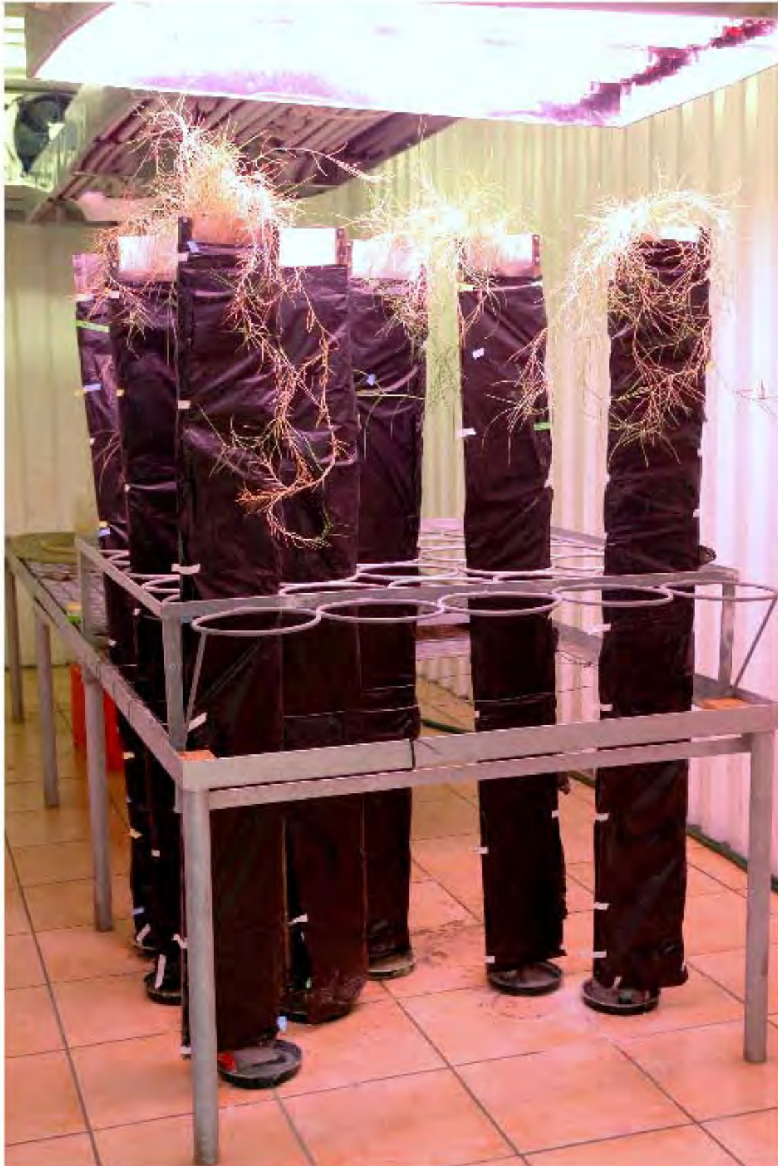
Figure 4.5. Columns used in the coal dump simulation study were placed upright and maintained in a constant environment chamber, as shown in the picture, and exposed to a temperature of 25°C and a day: night light regime of 16:8 hours. Cynodon dactylon was planted in the surface layer and columns watered daily.
