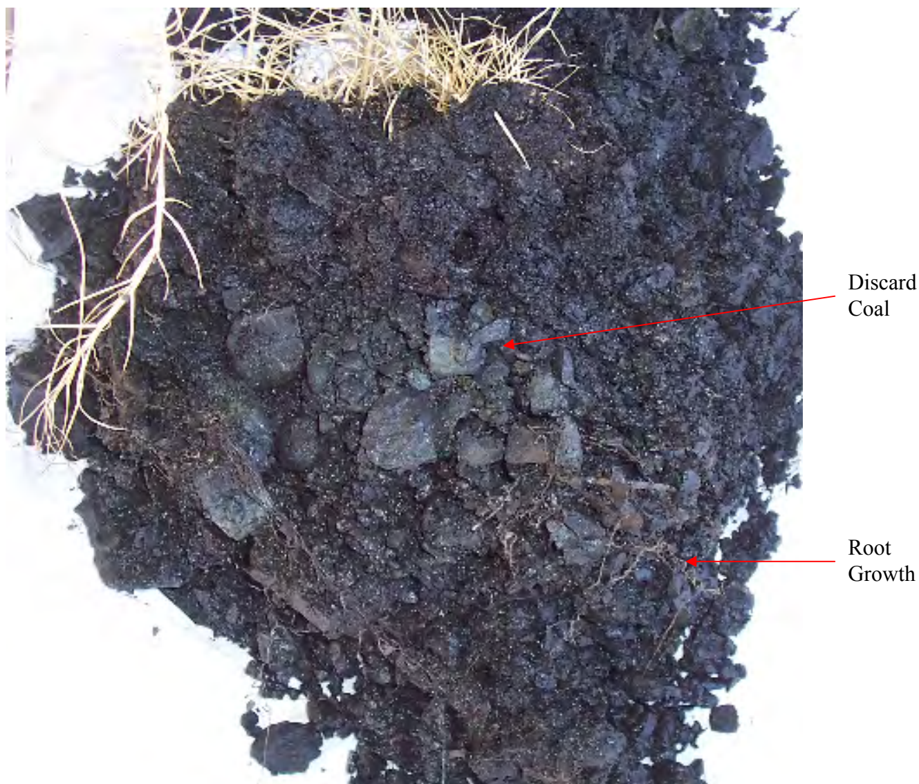
Figure 2.3. At harvest, it was observed that root growth in treatments involving hard coal amended with a weathered coal supplement was reduced in comparison to where soil cladding was utilised. The contents of a treated pot (HC + WC + C.dactylon ) including root growth within the discard coal can be seen in the picture.
