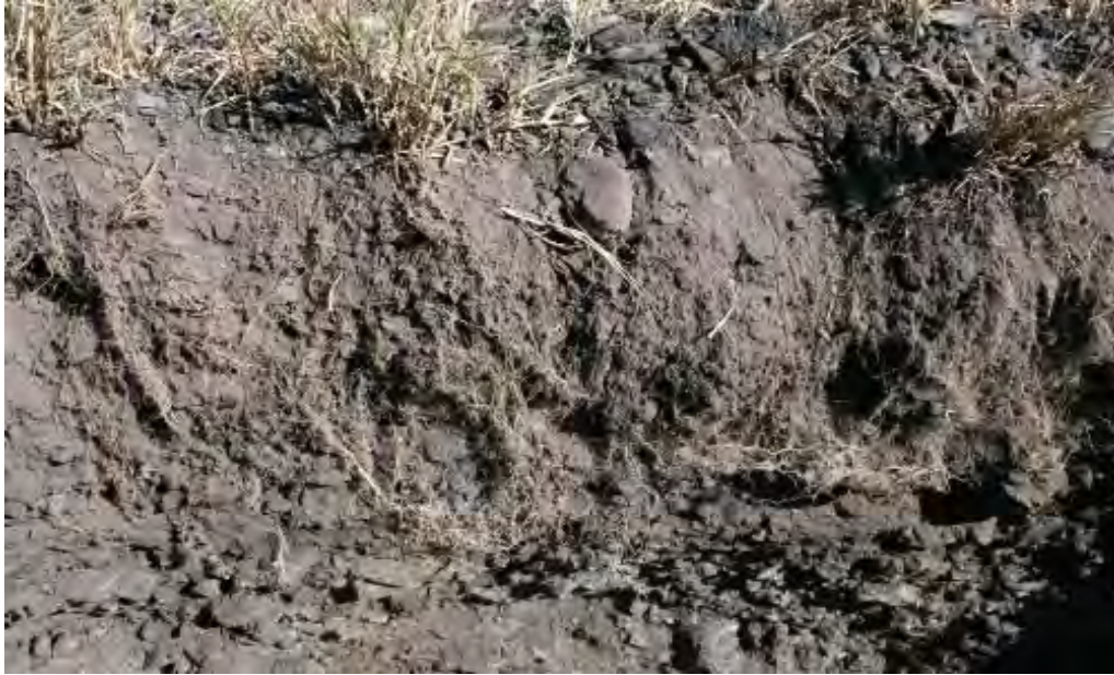
Figure 1-6 Cross section of a hard coal discard dump that has been transformed into a soil like material through the interaction of Cynodon dactylon and associated fungi at Navigation Colliery dump site (Mpumalanga, South Africa). The field of view is 45 – 50 cm
