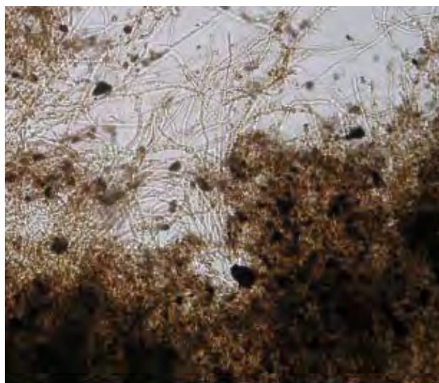
Figure 7-5 Micrograph (x40) of geologically oxidized coal adsorption onto the surface of N. fischeri pellets.
