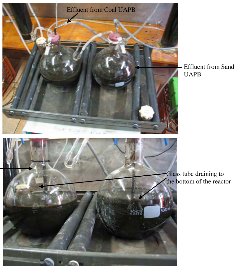
Figure 6-4 Experimental set up of the flask reactors for external extraction of HA from oxidized hard coal using alkaline effluent collected from coal and filter sand reactors.
