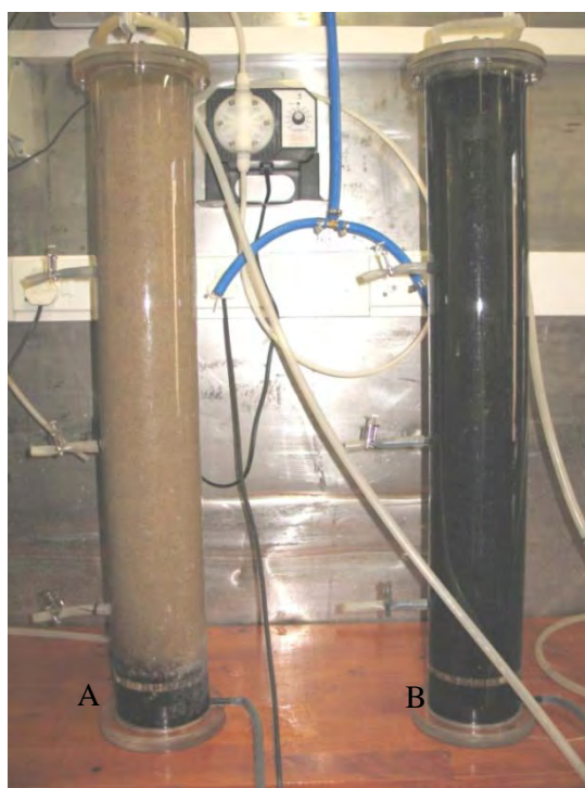
Figure 6-3 Experimental set up of the up-flow anaerobic packed bioreactors used in the investigation of humic acid as the carbon source for sulfate reduction in the presence of a co-substrate. Sand packing (A) and roof coal packing (B).
