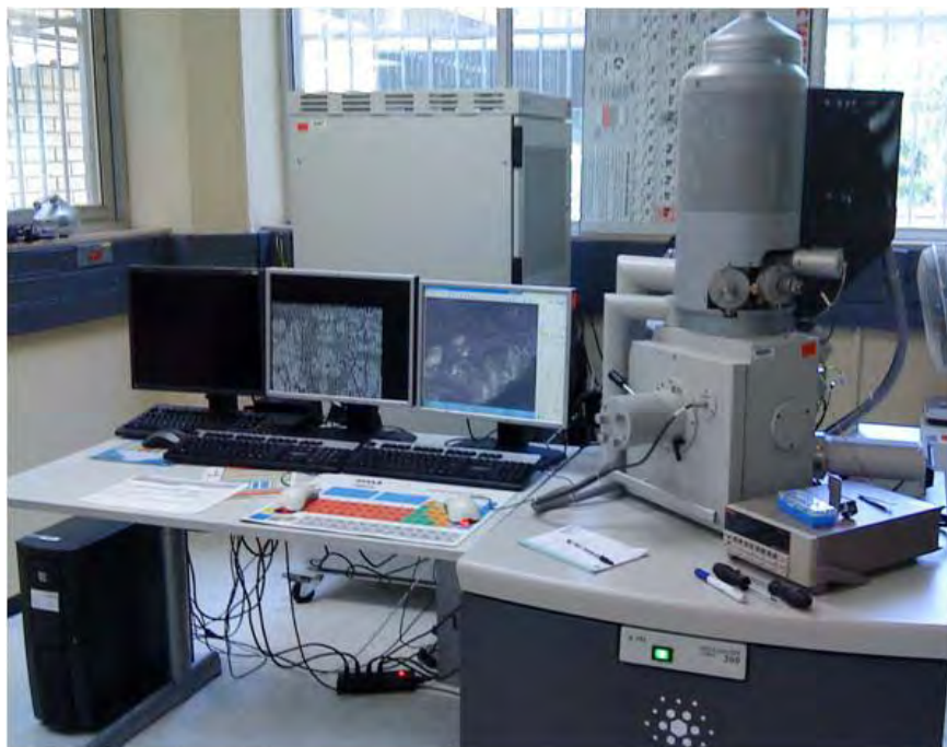
Figure 2.13 The FEI Nova 230 High resolution scanning electron microscope setup utilized in this study.
