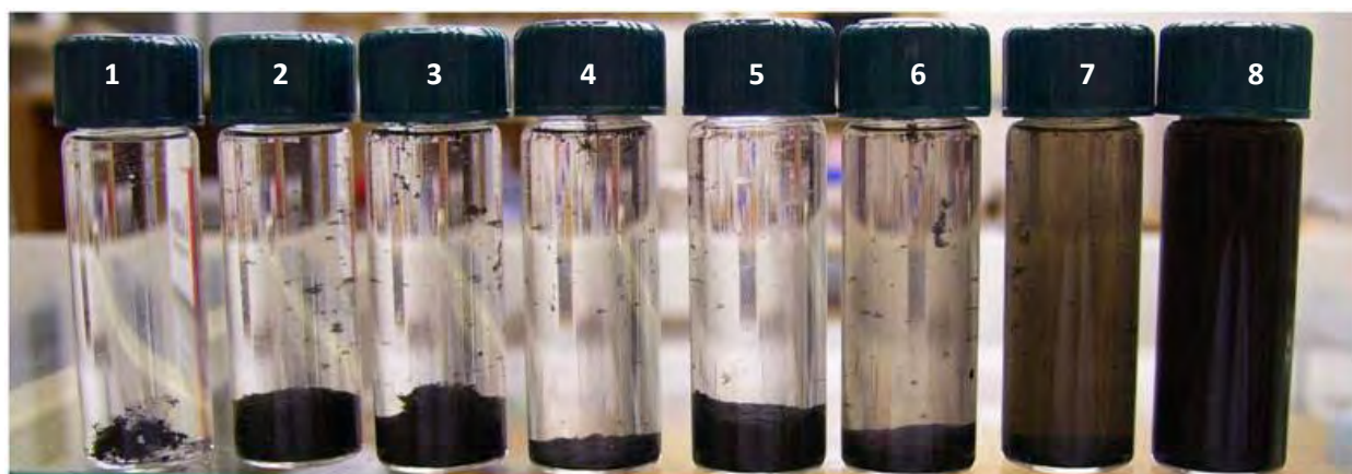
Figure 4.2 Functionalisation of SWCNTs: sample vials showing samples of single-walled carbon nanotubes (each suspended in 4 ml dH_2O ) taken at each hour and rinsed in dH_2O . On the far left is the vial following 1 hour treatment, whereas the far right hand side is the sample at 8 hours. Note: each sample is 5 ml total volume and was aliquoted from the same reaction vessel at hourly intervals. Discrepancies in observed volumes of precipitated nanotubes could be attributed to variances in density between the different functionalisation times.
