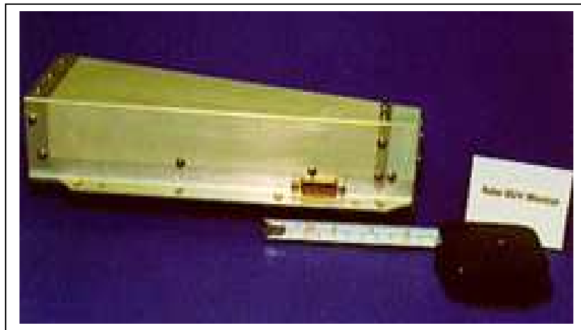
Figure 2.7: Image of SOHO Charge, Element, and Isotope Analysis System/Solar Extreme Ultraviolet Monitor instrument ( http://www.usc.edu/dept/space_science/instrument_pages ).
