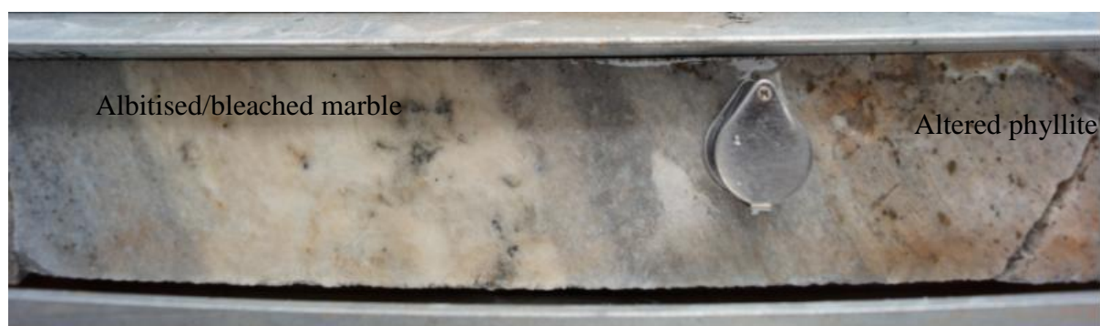
Figure 45. Bleached Albite alteration zones in LM. KRDD (29.90-34.50)
