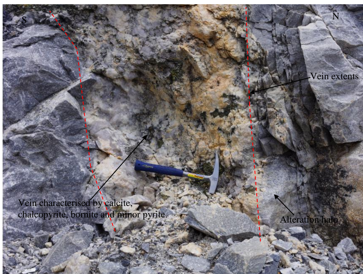
Figure 37. Carbonate-sulphide-rich veins in the Main pit, dominantly consists of chalcopyrite, bornite and minor pyrite hosted in schists of the LCS (looking west).
