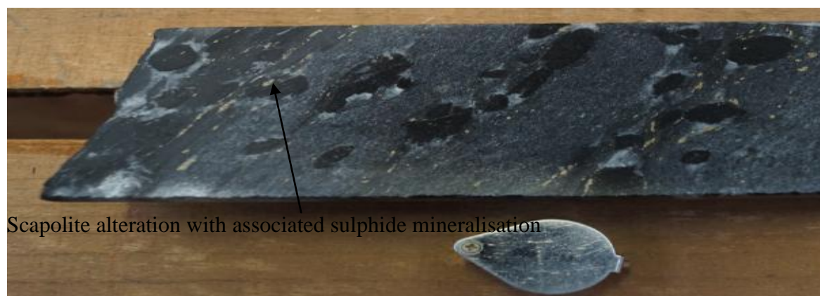
Figure 48. Scapolite alteration associated with sulphide dissemination (Py) in marble. KRDD455, 326m
