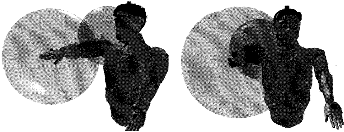
Figure 4.8 Intersection of the two spheres in a circle. The spheres each have as centre the shoulder and the wrist and as radius respectively the upper arm and the forearm. The elbow always lies in the intersecting circle (in white). The blue cubes represent the positions of the trackers.
