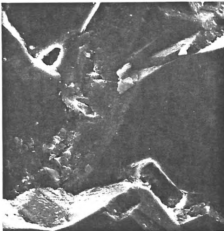
PLATE 5 : Note presence of silicate "plates" and 2 possible etch pits.
