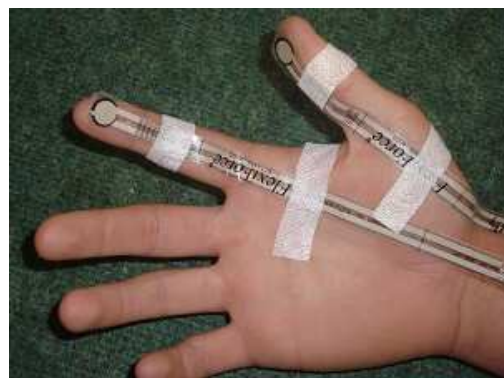
Figure 3: The placement of the pressure sensors on the first and second digits during the tactility test.
