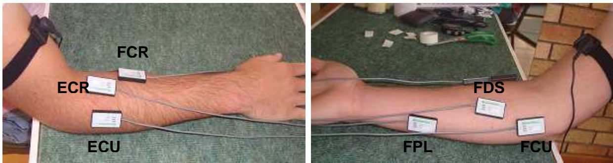
Figure 7: Electrode placement from left to right: ECR, ECU, FCR, FPL, FDS, and FCU.
