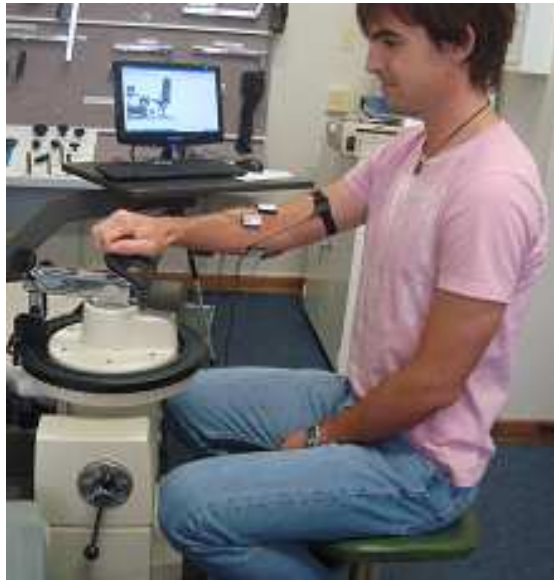
Figure 9: The participants' posture, and the dynamometer set-up during the torque test.
