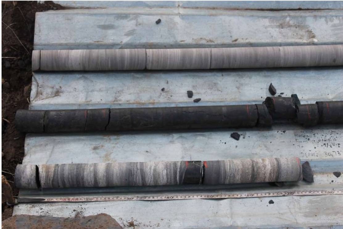
Figure 16. Borehole core ready for logging.
