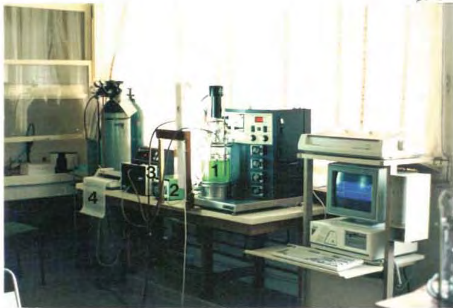
Plate I The experimental equipment used in the fluorescence-quenching study. 1=Bioflow III Reactor; 2=Peristaltic Pump; 3=Fluorometer; 4=Chart Recorder
