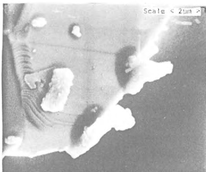
Micrograph 28. Copper(II) oxide conditioned with Oxine for 2hrs at pH 3,5.
