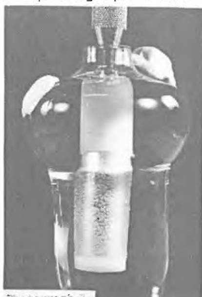
Photograph B. Subsequent growth of \text{Cu}(\text{Ox})_2 on copper metal.
