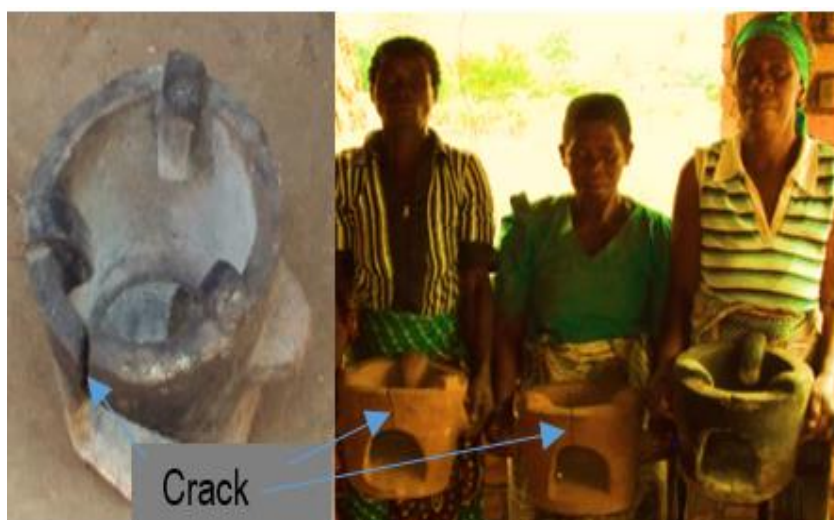
Photo 6.1: Stoves with a crack on the upper door of the stove from Chapita Village in Balaka district, and Mvuduma Village in Mulanje district (Chisoni, August 2014)
