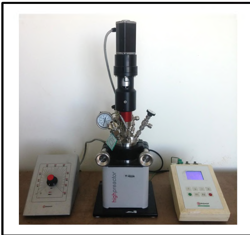
Fig. 2.1. Berghof high pressure reactor employed for the hydrothermal syntheses of the GQDs/gCNQDs used in this work.
