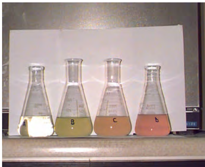
Figure 3.2. Picture showing brine samples collected from: A- Inlet; B- E2; C- E5; D- X2. Reflection in sample A occurred due to the clarity of the brine.
