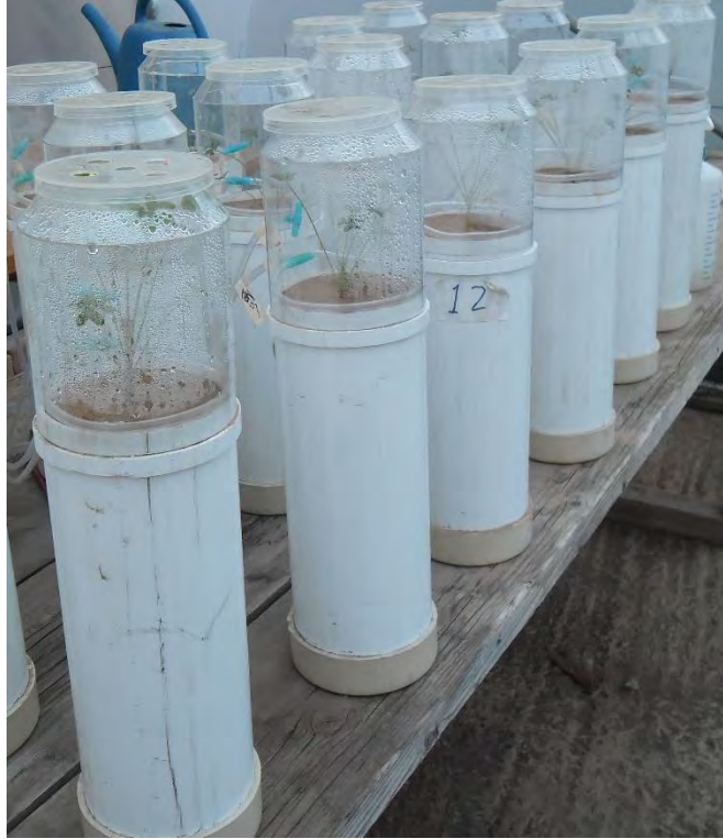
Figure 2:1: Custom-made mini open top chambers used to grow Oxalis pes-caprae and O. punctata to study the effects of glacial CO 2 concentrations.
