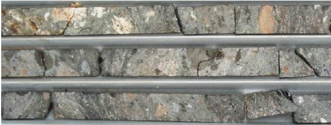
Fig.13. Polymictic axial breccia showing angular clasts of siltstone, dolostones, shale and sandstone (picture from Jigsaw, 2009, unpubl.)
