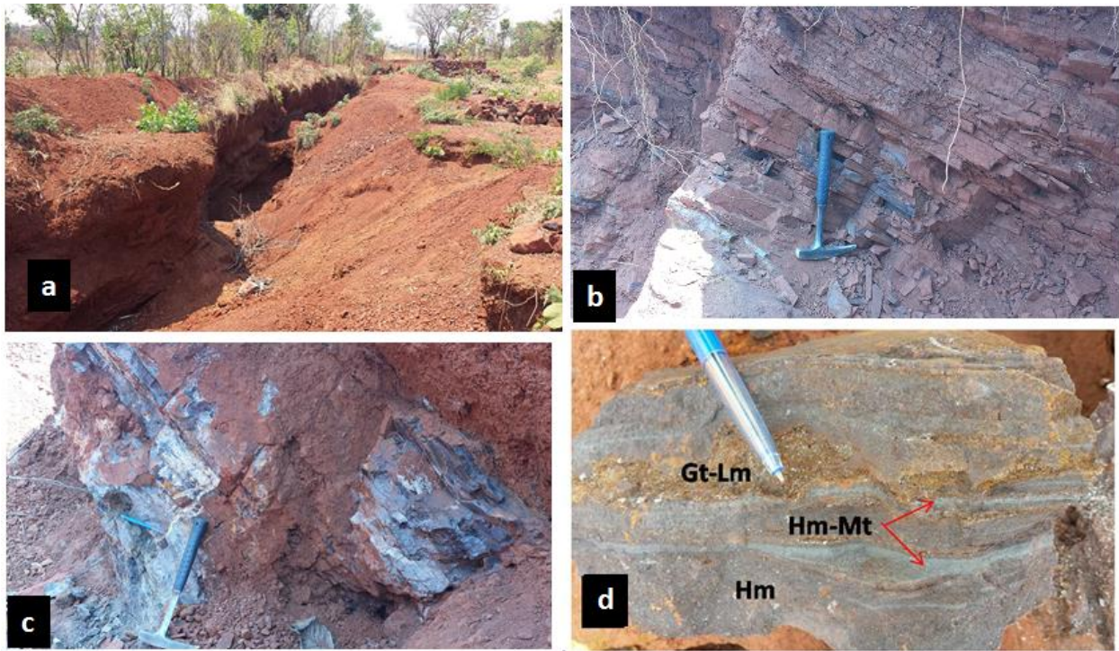
Fig.12. Iron formation outcrops: (a) local diggers pitting along iron formation; (b) NE dipping banded iron formation; (c) brecciated and enriched iron formation associated to whitish carbonate veinlets; (d) layering composition of the iron formation showing magnetite (metallic), hematite reddish metallic, goethite and limonite (yellow). Note Gt=Goethite, Hm=hematite, Lm=limonite, Mt=magnetite;
