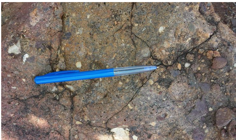
Fig.14. Ferruginous matrix of polymictic axial breccia, outcropping in Nakarimba area
