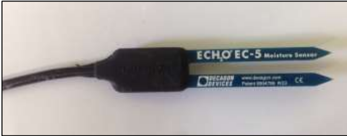
Figure 15: EC-5 soil moisture probe (8.9cm by 1.8cm).
