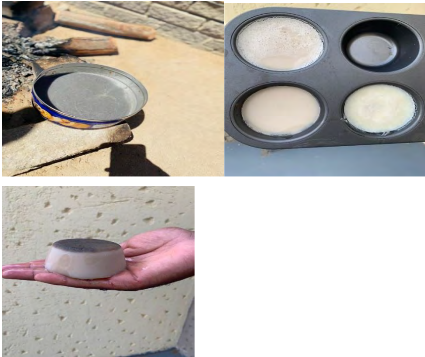
Figure 6.15: Shows the liquid soap poured into a moulding container for it to solidify
