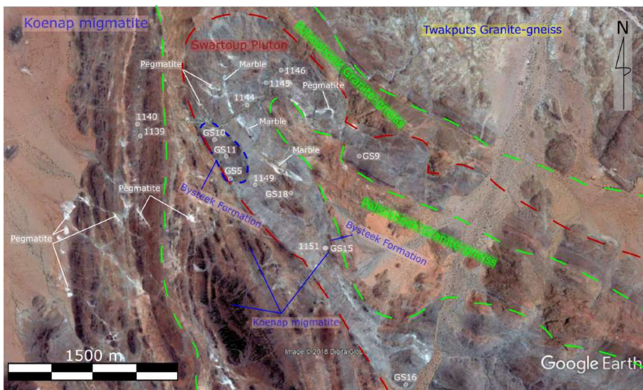
Figure 3.6: The satellite image shows investigated localities of the Swartoup Pluton. Notice the proximal relationship of garnet-bearing granitoids (1140A, GS15C, GS16A) to Koenap migmatite outcrops, and of pyroxene-bearing rocks (1151A, GS15B, GS10B) to Bysteeek Formation. The specimens comprising the geochemically distinct group Swartoup 1 were collected in the north of the study area. Samples 1139A and 1140A were sampled from a dyke to the west of the Pluton, surrounded by Koenap Formation. Samples 1144A, 1145A and 1146A were collected nearer the hinge of the antiform (image ©2018 Google).
