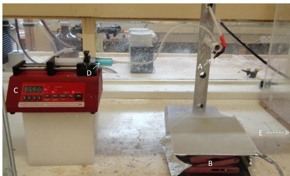
Figure 5.1: The electrospinning setup used in the present study. A: metal needle (inner diameter: 0.3 mm) connected to the positive voltage supply, B: collector (covered with aluminum foil), C: pump, D: Syringe (containing polymer solution), E: voltage supply. This image was obtained using a SONY Cyber shot digital camera.
