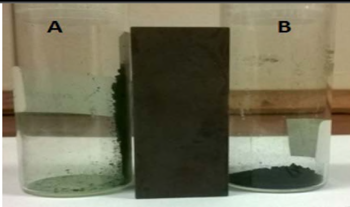
Figure 3.12 Photograph of the 10-MNPs (A) and 10 (B) exhibiting magnetic property of the former
