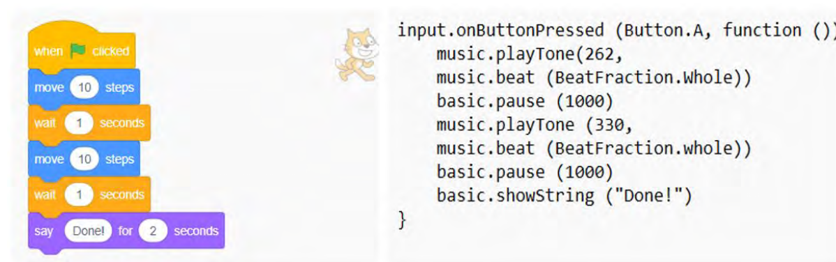
Figure 1: Similar programs in two programming environments. (left: Scratch(visual), right: Javascript in Micro:bit(text-based))
