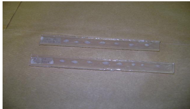
Figure 5.12: Photograph of otoliths (the sagittae) of Hydrocynus vittatus sp. (a) The otoliths are retrieved from the skull of the fish. (b) The otoliths set in a casting resin rod ready for sectioning.
