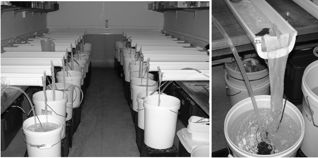
Figure 2.7: Artificial stream systems or channels used for organisms collected from lotic environments
