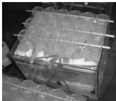
Figure 2.9: Lentic experimental system – aerated glass tanks with individual 50ml plastic vials (suspended on wooden dowel sticks) to accommodate predacious organisms
