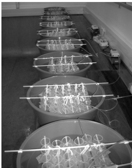
Figure 2.10: Lentic experimental system – aerated plastic tubs containing 40+ 50ml plastic vials suspended by string on wooden dowel sticks
