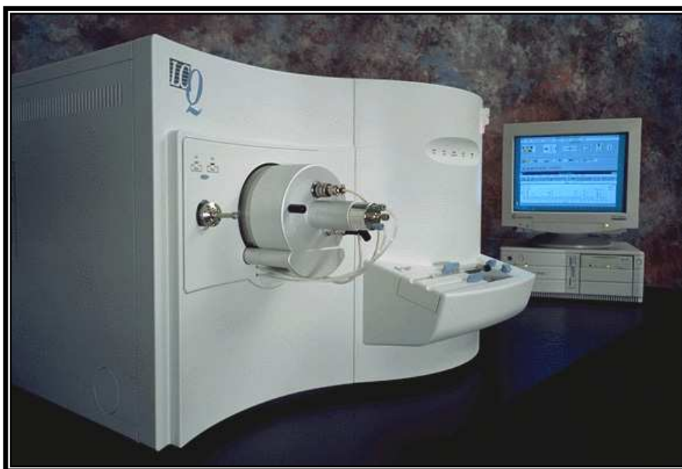
Figure 6.5: Photograph of the Finnigan LCQ system equipped with an atmospheric pressure chemical ionization (APCI) source.
