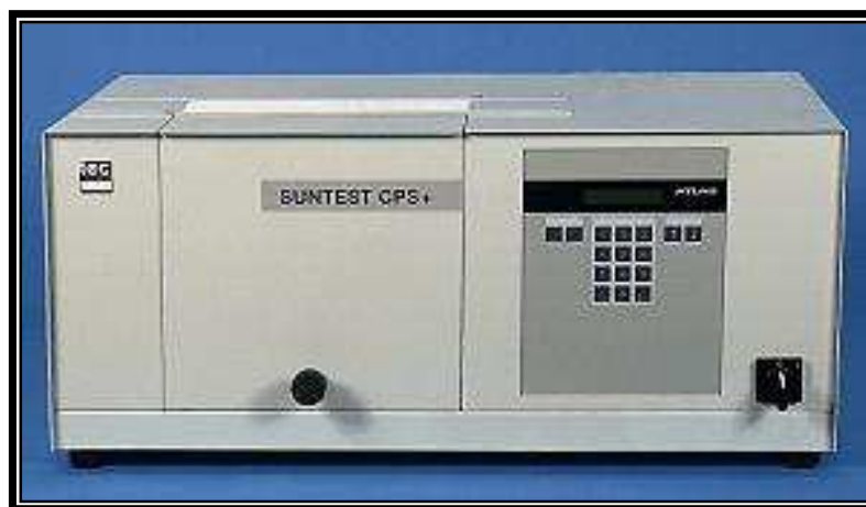
Figure 5.3: Photograph of the Hereaus Suntest CPS+ (ATLAS, Gelnhausen, Germany) used to irradiate the melatonin samples according to ICH guidelines.
