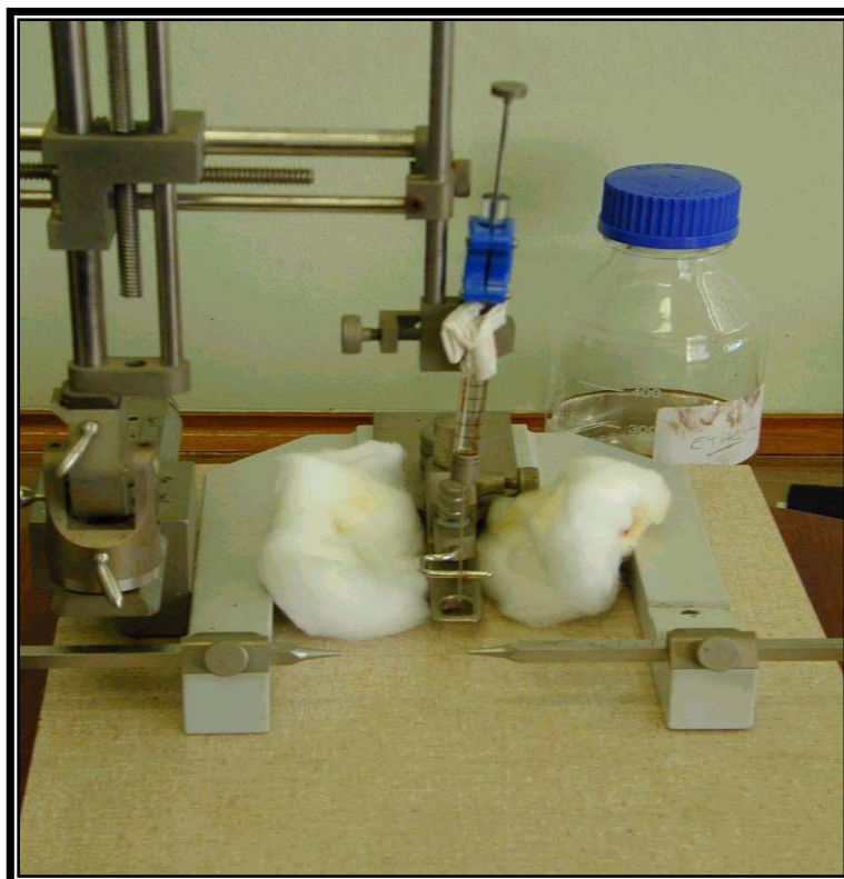
Figure 8.9: A view of the stereotaxic apparatus and Hamilton syringe used for the bilateral intrahippocampal injection of QA (Stoelting, IL, USA).
