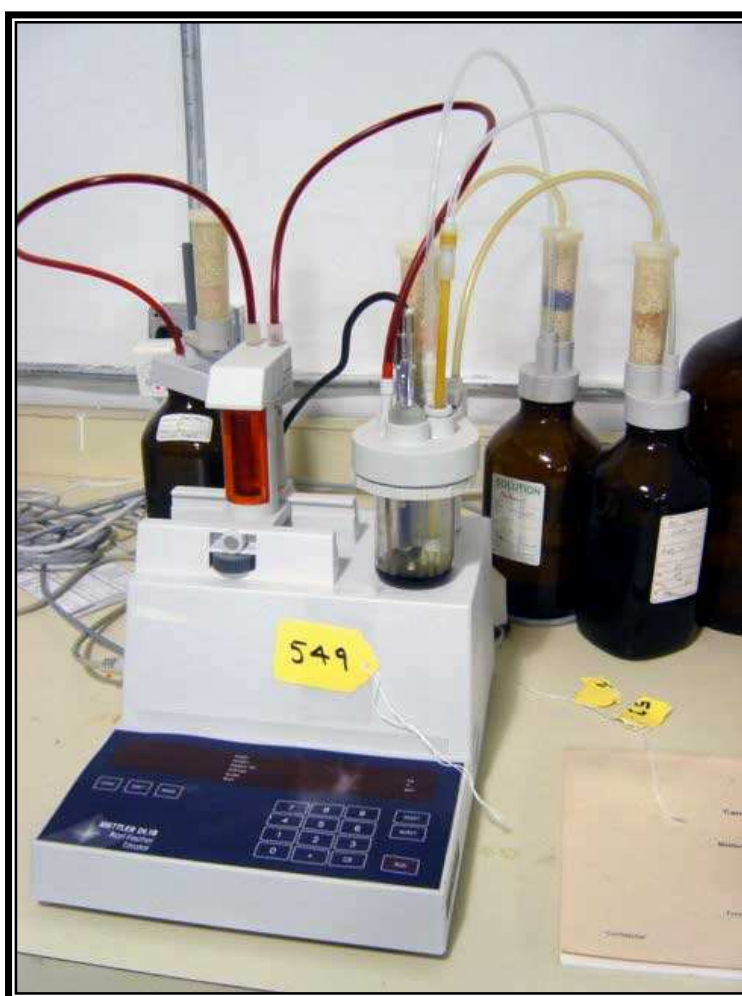
Figure 3.12: Photograph of the Karl Fischer Titrator Apparatus (Mettler DL 18).
