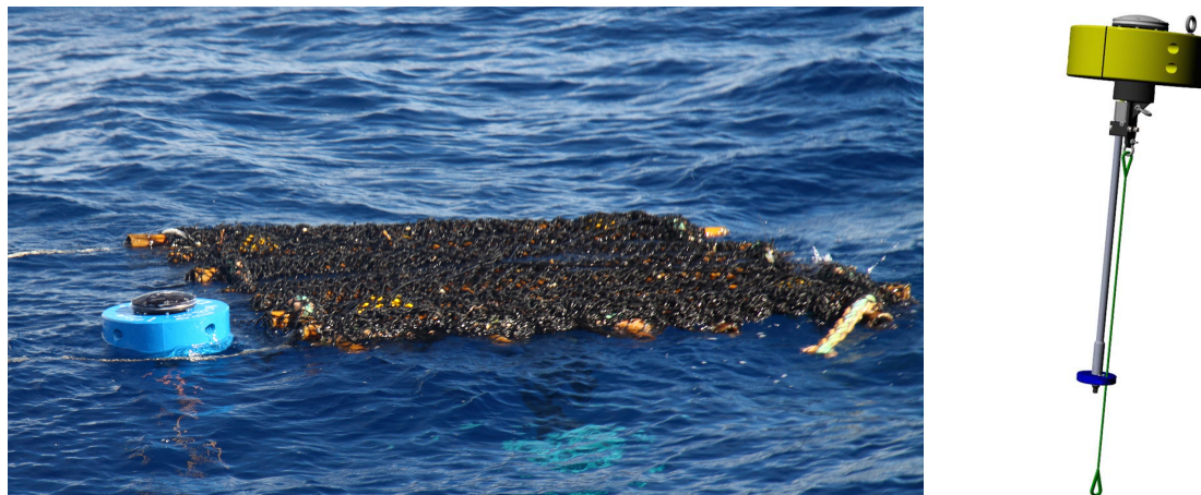
Figure 2.4 VR4-Global acoustic receiver attached to a drifting FAD (left) and a schematic diagram of the receiver unit showing the submerged part with the hydrophone (right).
