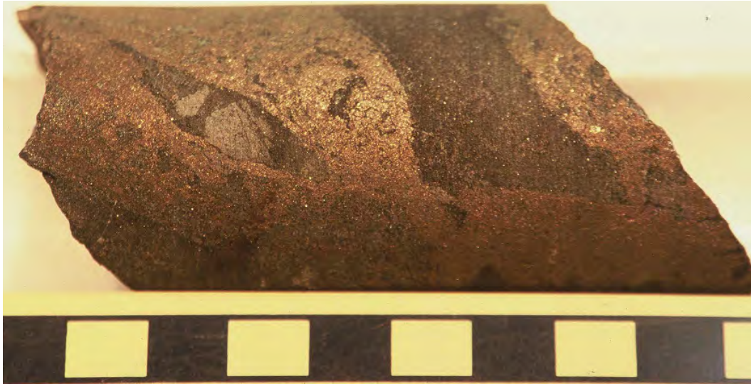
Figure 2.43: Massive sulphide sample with clasts of amphibolite containing quartz vein material. (Sample R7-22).
