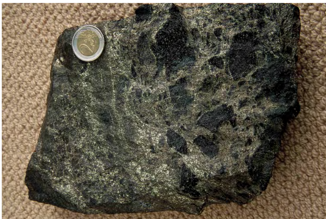
Figure 2.42: Massive sulphide sample from Peltosaari. Clasts of coarse biotite-rich rock. The principal sulphide present is pyrrhotite with lesser amounts of chalcopyrite, molybdenite and pyrite (Diameter of coin is 26 mm).
