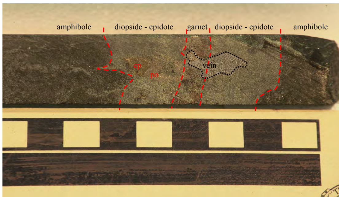
Figure 2.34: A zoned calcic-skarn vein in amphibolite. A fragment of a discontinuous quartz-carbonate vein is surrounded by a rough alteration halo with a core zone of garnet, passing into a diopside-epidote zone and finally into an amphibole zone. Large blebs of pyrrhotite and chalcopyrite are also present (Sample R8-169).
