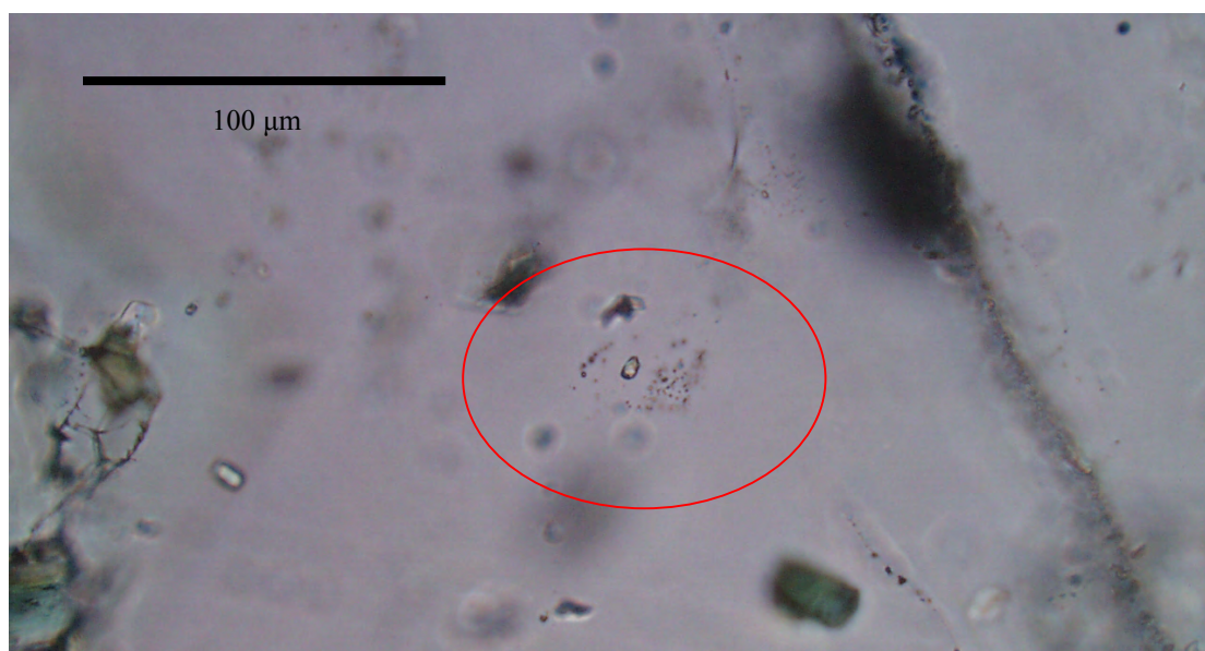
Figure 3.47: Photomicrograph of a decrepitated fluid inclusion from sample R8-219. The three-dimensional cluster of small secondary inclusions surrounding the parent inclusion, is an implosion texture resulting from isobaric cooling (Vityk & Bodnar, 1995).
