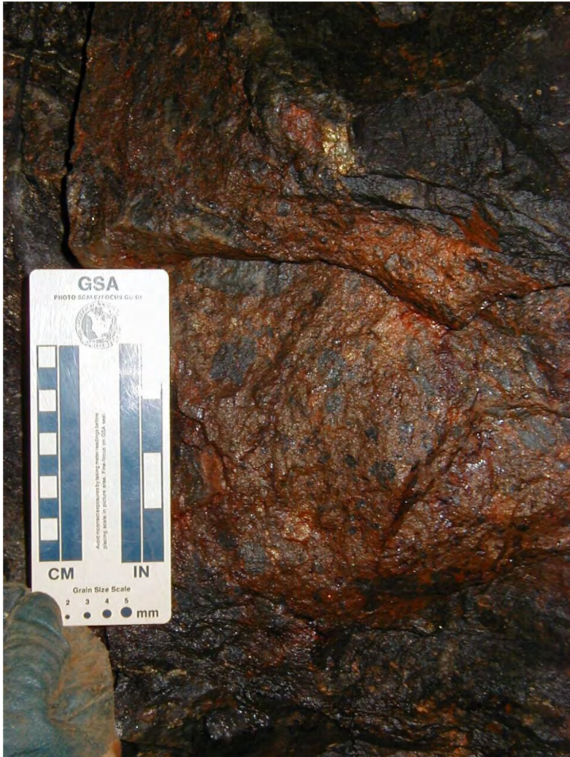
Figure 2.45: Massive sulphide / cataclastite with rounded clasts of vein quartz. Photograph taken underground at the Haveri mine.
