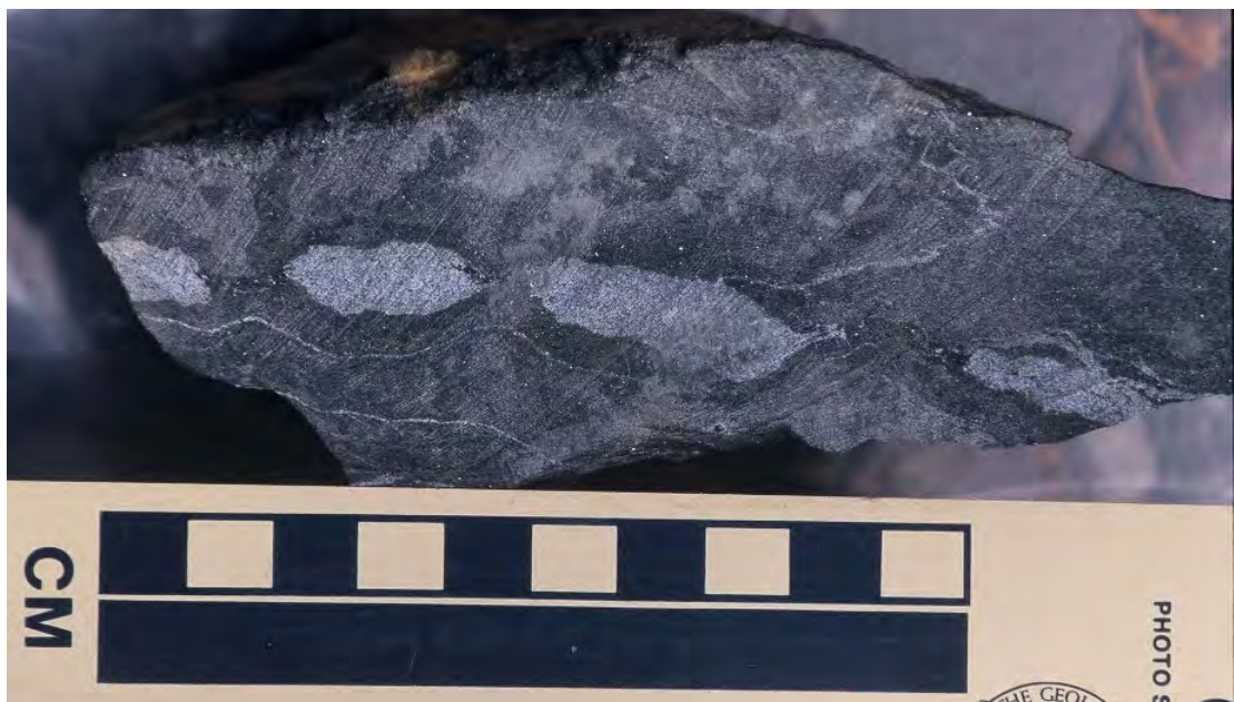
Figure 2.38: Boudinaged quartz vein, with a rim of amphibolitisation. Sample from underground in the Haveri mine.
