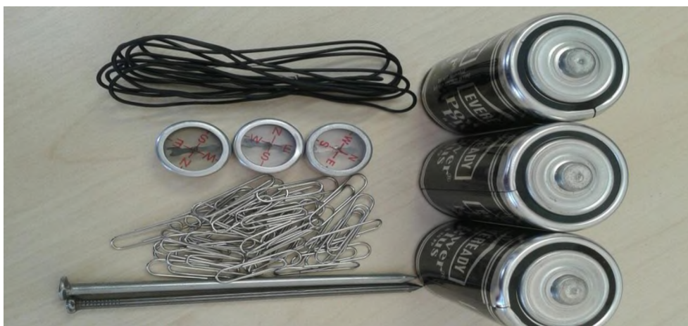
Figure 4.3: An electromagnetic kit made from easily accessible materials for a group of about 4 learners
