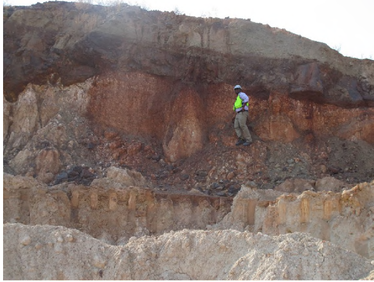
Figure 8: Main magnetite Layer (MML) at Glencore's Rhovan mine. Notice the variable thickness of MML at the the outcrop scale, as well as the limonitized non-planar anorthosite floor of the MML
