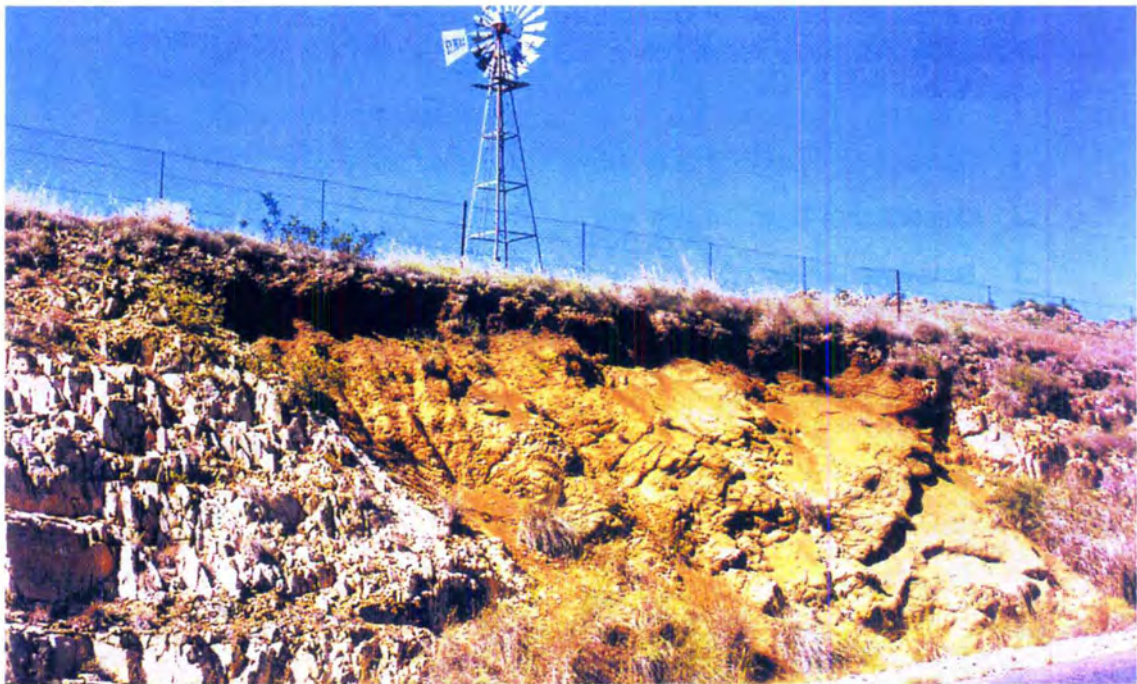
Plate 3: A borehole targeting a highly fractured sandstone aquifer at the margin of a dolerite dyke (weathered light yellowish brown).
