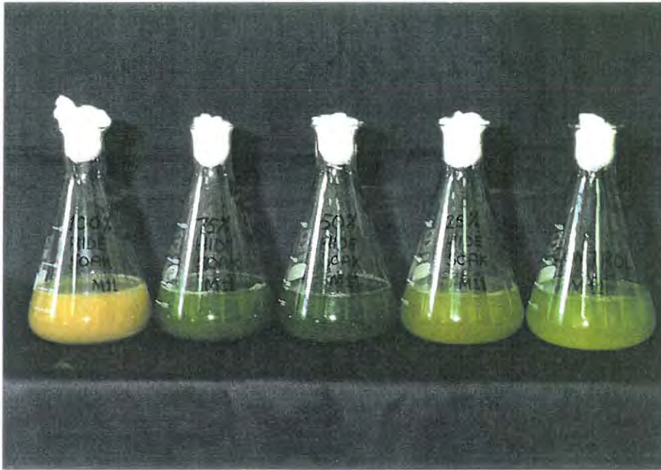
Plate 6.1. Growth of Dunaliella in a range of hide-soak effluent strengths (from left to right: 100%, 75%, 50%, 25% and control).
