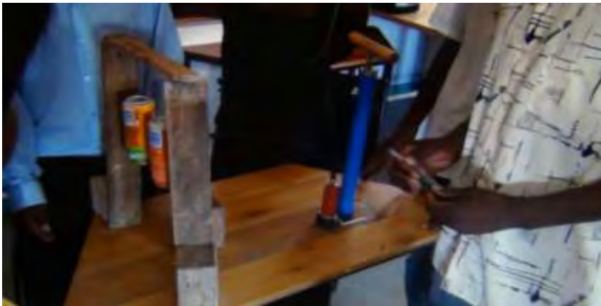
Trainer teacher uses a bicycle pump to blow air between the suspended cans
