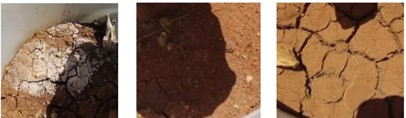
Figure 2.19 Images of the soils twelve weeks into the experiment. From left to right soils were subject to irrigation treatments: constructed wetland, nutrient solution and water.
