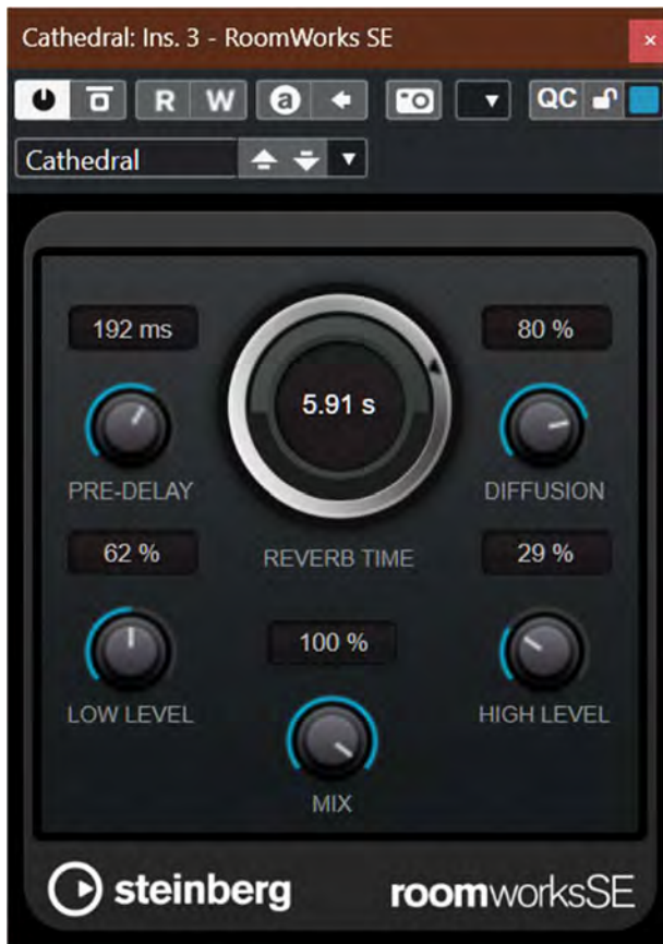
Image 6.7.2: The image shows the parameters of the cathedral reverb preset by RoomWorks SE.
