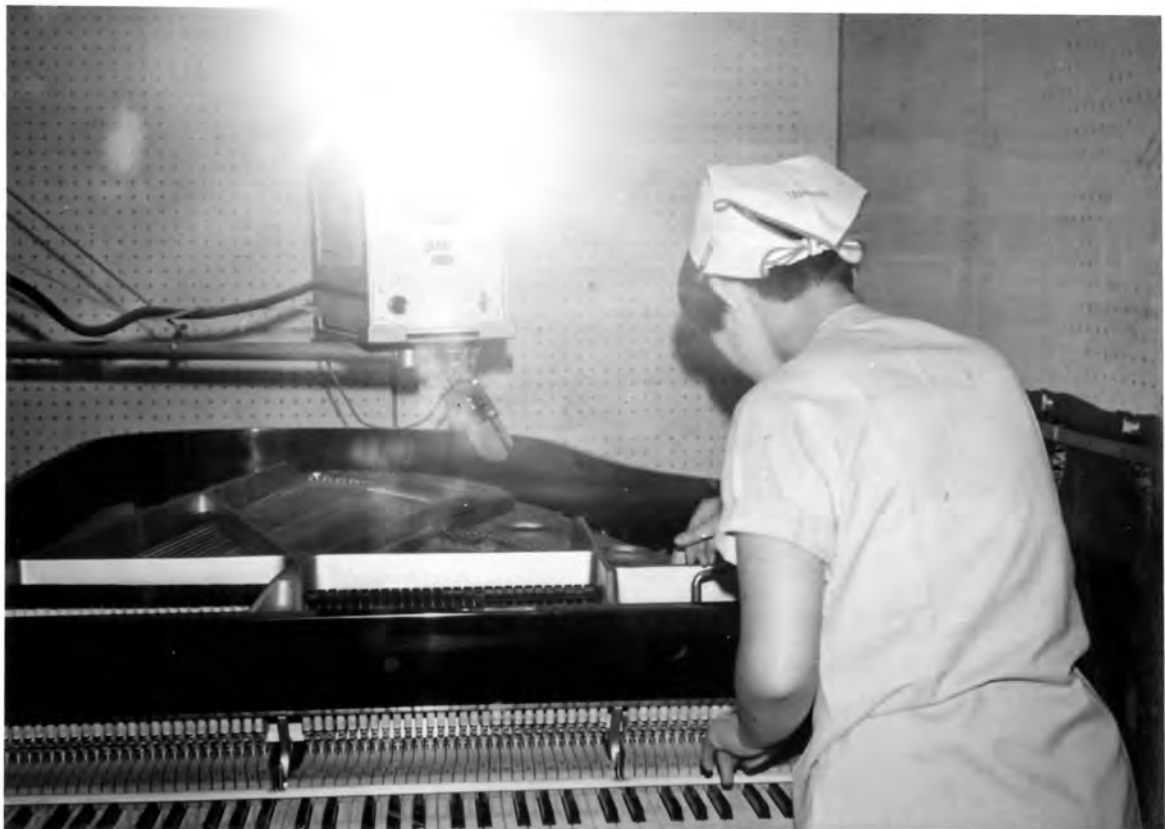
Tuning using an electronic aid, Nippon Gakki Company, Hamamatsu. The operator works in a soundproof glass fronted cubicle. Photo by writer 1970.
