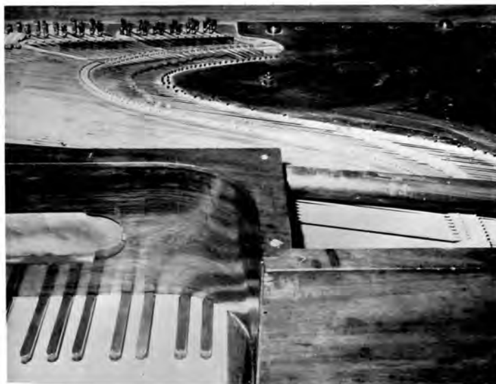
View of Collard & Collard (11870) showing rounded black keys. The method of using one string fixed to two wrest pins and looped over the hitch pin, can be seen in this picture.
