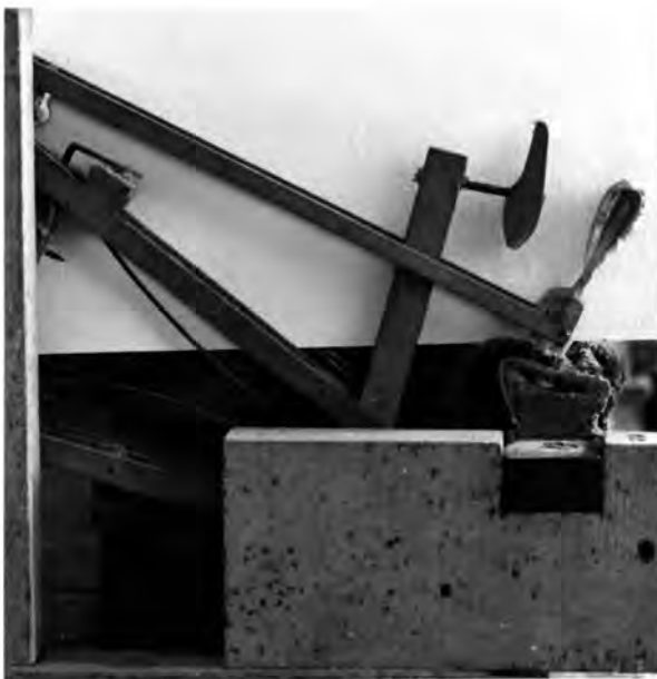
Action of the Erard Grand at Kingswood College showing hammer in rest position and with the key depressed.
