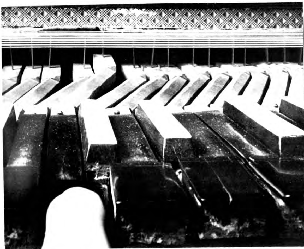
The picture depicts a player depressing Middle C on a Clavichord. The tangent at the far end of the key lever has been raised so that it has struck the strings and has lifted them above rest position. The damping cloth on the left of the raised string can also be seen.
