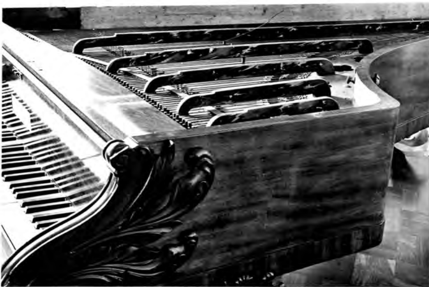
View of Harper piano showing the narrow metal strip screwed down over the strings - a type of Capo Tasto bar.
