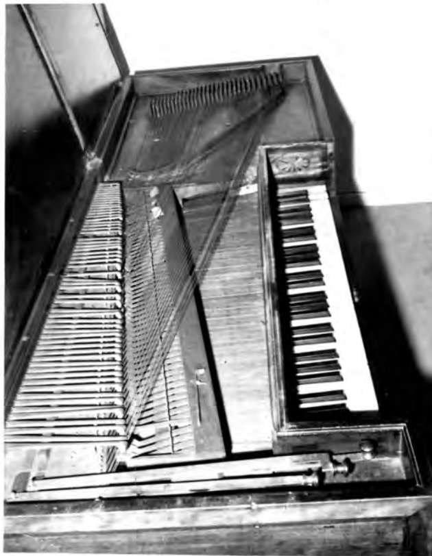
Plan View of Adam Beyer Square showing overdampers and three hand levers. L - R: Damper for Treble notes, damper for bass notes, lute (sourdine). A damper can be seen lying on the hammer rail. Action described in Fig. 39. Note the wrest pins on the right of the soundboard.
