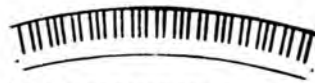
6. THE CLUSAM KEYBOARD, curved and concave, taking account of the fact that the arms move in arcs on two planes
