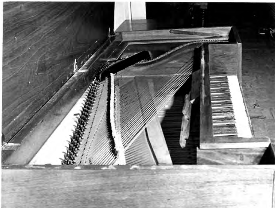
Broadwood Square (04 883) showing the metal hitch pin plate and transverse bracing bar. Action as in Fig. 39.
