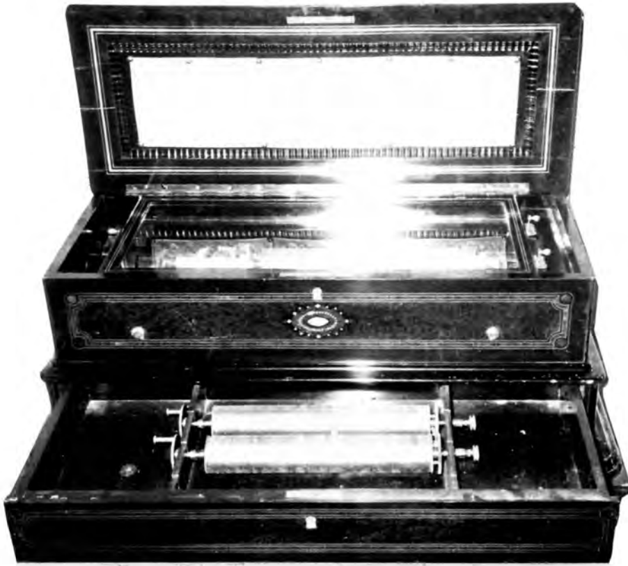
Musical box in possession of Mr. F. White, Grahamstown. The open drawer shows two of the three cylinders. An index of tunes is pinned onto the lid and a hinged glass lid covers the mechanism. The measurements are 33\frac{1}{2} " wide x 14" deep x 18\frac{1}{2} " high.
