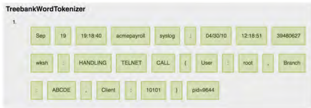
Figure 2.4: Tokenization using a Treebank Tokenizer tokenization (Perkins, 2018)
