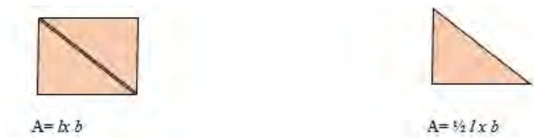
Figure 2.1: The area for a right-angled triangle is half the area of its rectangle
