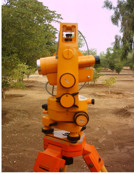
Figure 3.3: MINGEO Zeiss 010 DI-flux non-magnetic theodolite, Abdus Salam Geomagnetic Observatory, Sonmiani. Image credit: Pakistan Space Weather Centre (PSWC).
