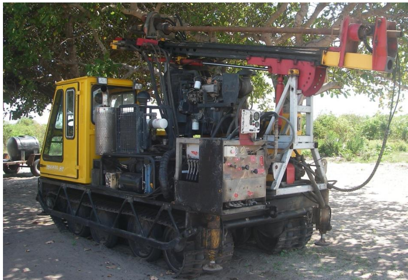
Figure 14: Picture showing the air core reverse drill rig used during the infill drilling in the Namalope deposit for thesis purpose.
