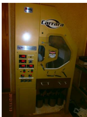
Figure 18: One of the magnetic separation machines used at Kenmare for magnetic and non magnetic separation of heavy minerals for XRF analysis.
