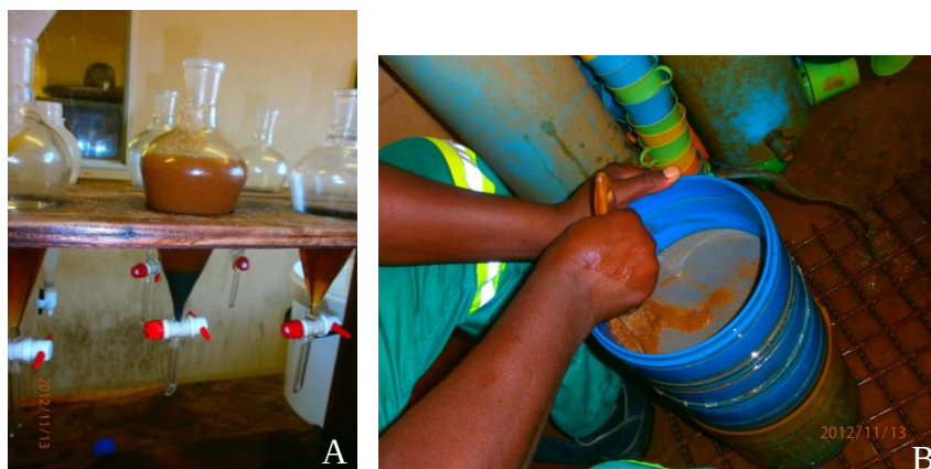
Figure 17: LST heavier liquid separation with heavier material at the bottom of funnel and lighter at the top in A and washing process of separate materials using paint brush in B.
