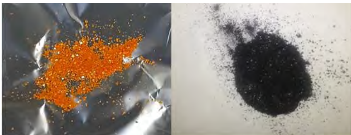
Figure 6.2: Image showing Ru_3(CO)_{12} before (left) and after placing in the oven (right)
