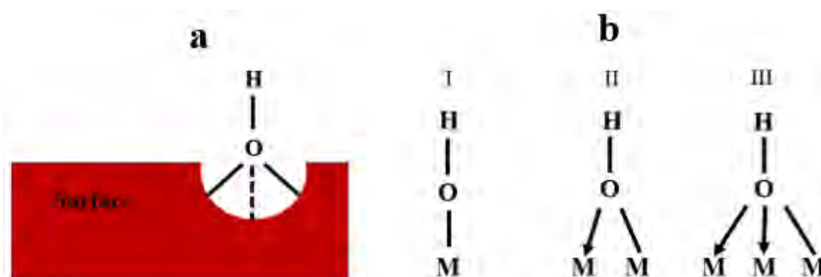
Figure 2.8. Interaction of water with oxygen vacancies on the surface of reducible metal oxides (a) hydroxyl formed as water dissociates over oxygen vacancies (b) types of hydroxyls formed, I is a terminal hydroxyl, II is a bridging hydroxyl with hydrogen coordinated to two metal atoms, III is a bridging hydroxyl coordinated to three metal 53 57
