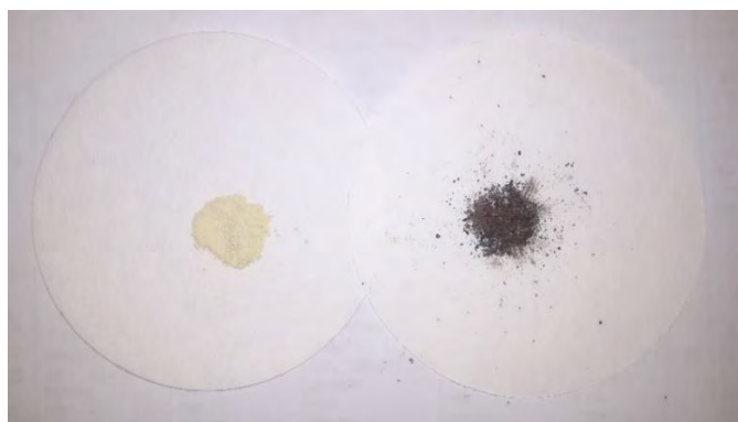
Figure 5.16: Image showing the colour change that took place on the catalyst during the reaction; Ni/TiO 2 before (left) and after (after) reaction at 200 °C as an example.
