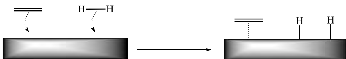
Figure 2.1. Illustration of how adsorption of molecules happens on a catalyst surface, using hydrogen and ethene as an example
