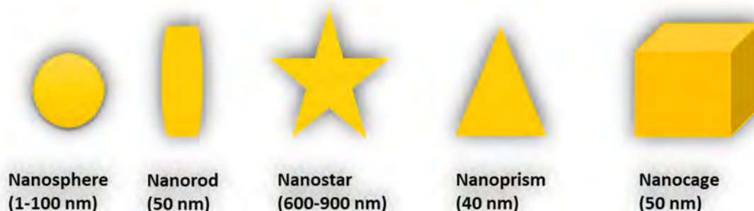
Figure 8. Gold nanoparticles of different morphologies and sizes.
