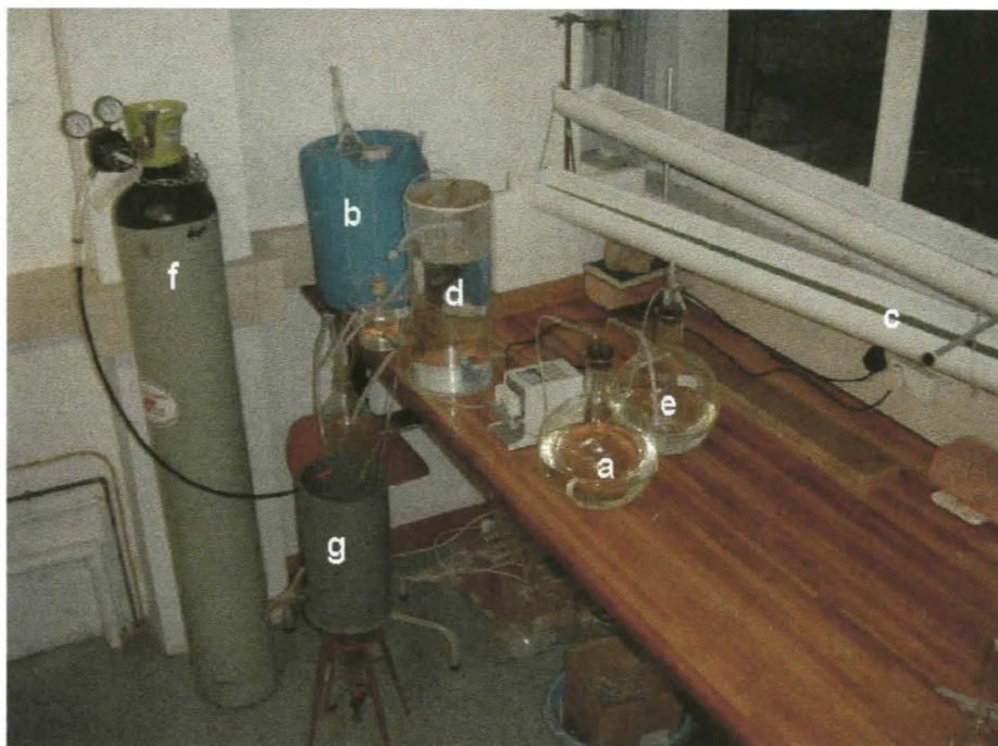
Figure 7.8: Bench scale integrated biological system showing the various components, a = anaerobic digester feed, b = 28l anaerobic digester, c = algal gutters, d = selective precipitation vessel, e = acid mine drainage, f = nitrogen source and g = precipitation vessel
