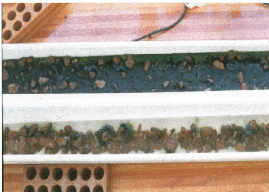
Figure 7.6: Seeding of the Oscillatoria culture in the simulated stream (gutter) reactors showing the adhesion of the algae to the solid supports and the subsequent extension of the filaments
