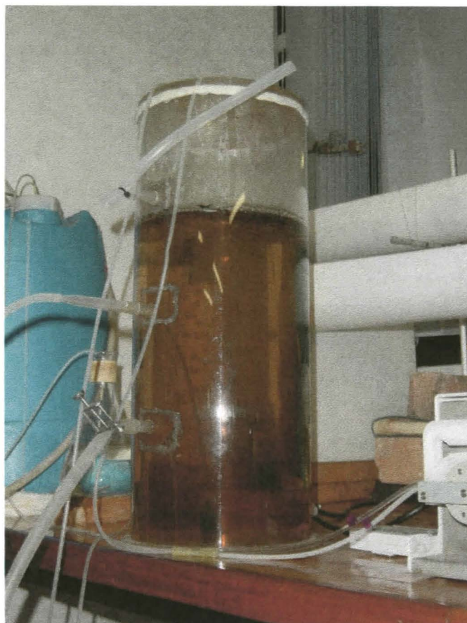
Figure 7.9: The selective precipitation vessel showing the formation of the brown copper and lead sulphide precipitate
